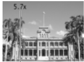
The combined magnifications of the optical zoom and digital zoom are displayed.
